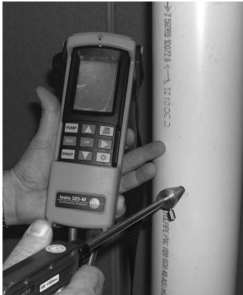
Figure 9.2: Insert Analyzer Test Probe into Test Port
